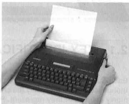
3. After the top of the paper appears, pull the paper release lever to release the paper and then align the top corners of the paper with the bottom.
