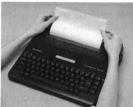
4. After the paper is aligned properly, return the paper release lever to its original position and move the top of the paper down by turning the platen knob.
